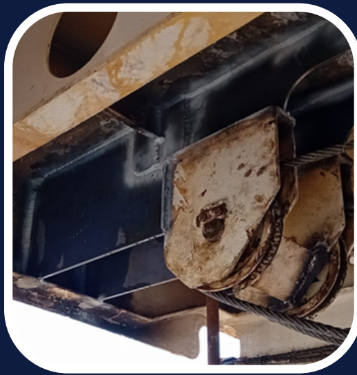
Photo 2 -New connecting plates for the pulley boxes
