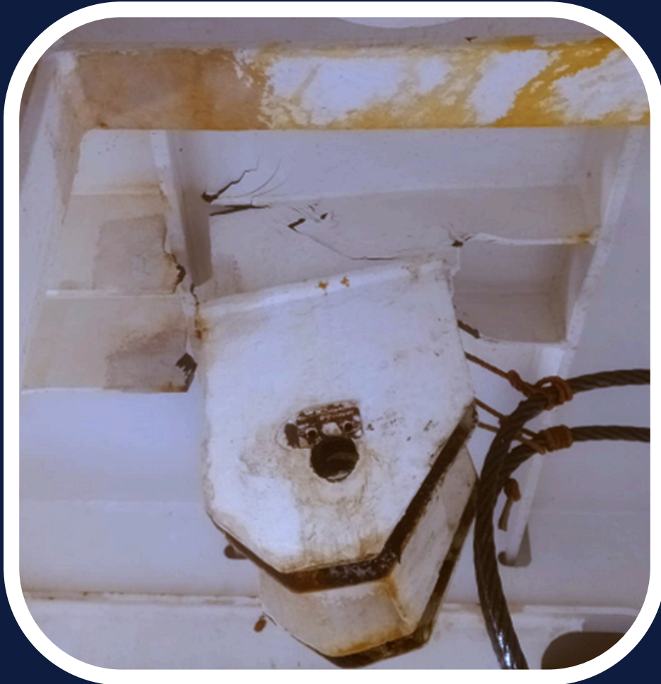
Photo 1 - Failure of the plates connecting the pulley boxes to the upper deck
