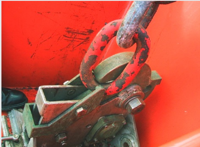
Photo n.2 An example of the incorrect (incomplete) master link insertion
