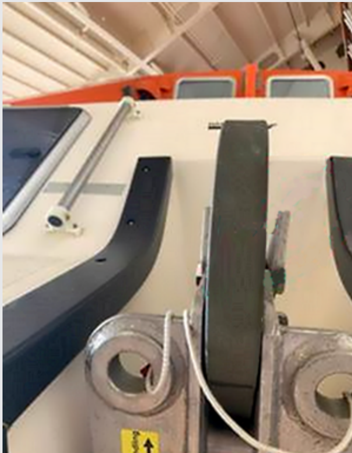
Photo n.1 The bent side-lid detected after the accident
