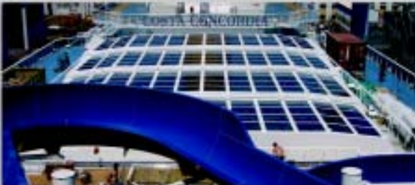
Machine Sliding Cover on Costa Concordia
