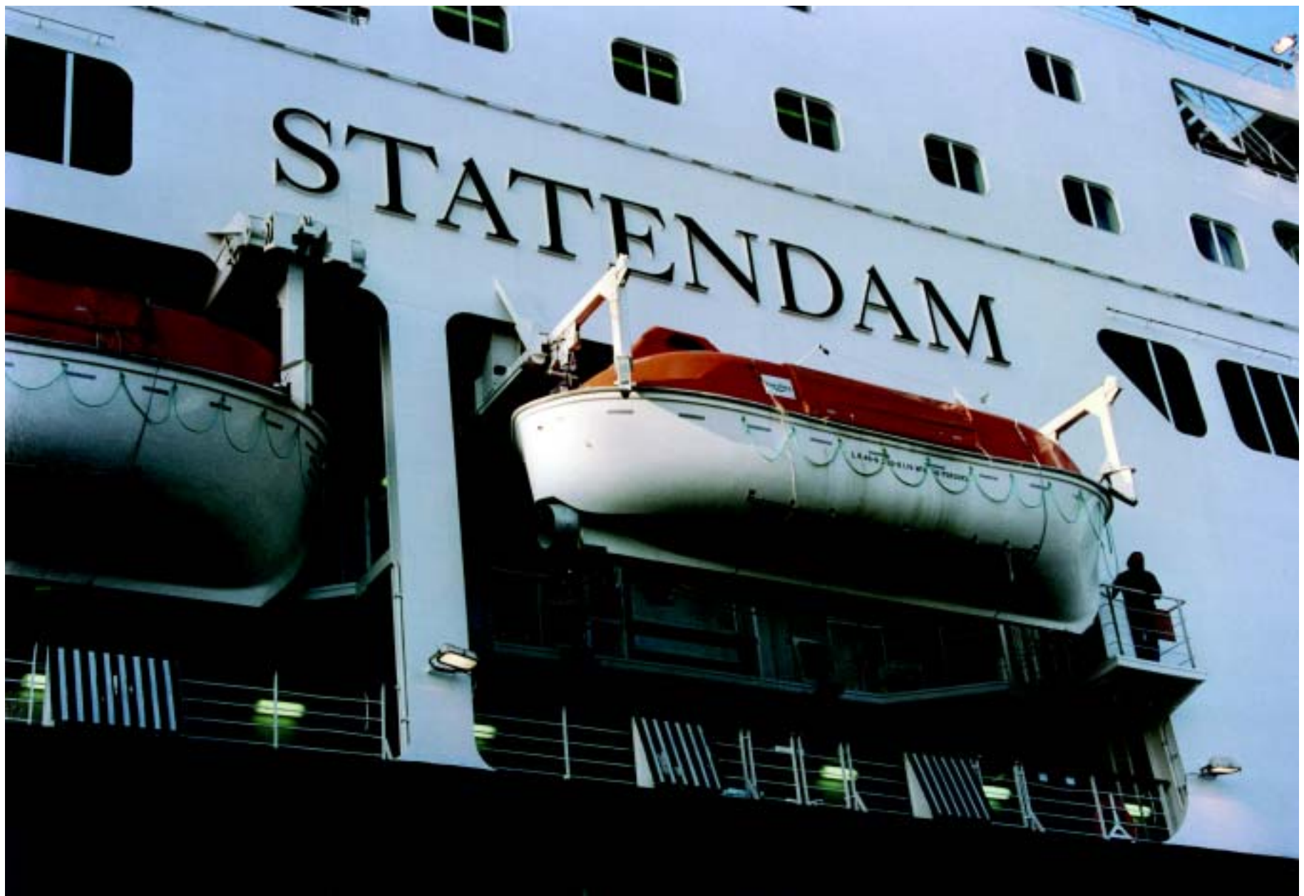
Statendam - First Telescopic Davits designed, manufactured and supplied by Navalimpianti Tecnimpianti
