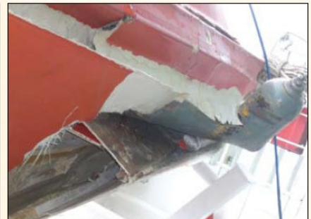
▲ Close-up view of damaged hull and ruptured air cylinder
