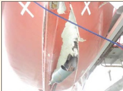
▲ View of damaged hull and ruptured air cylinder
